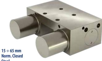
Working type Body Steel Operating Temperature 20°C ÷ +80°C Operating Pressure 5,5 ÷ 8 bar Switching time 40 ÷ 60 mSec Contact parts Hardness 60 ÷ 62 HRC
