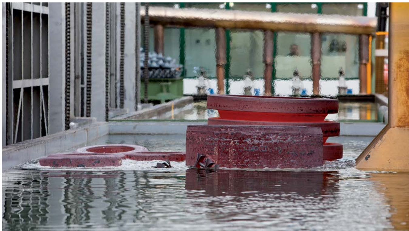
Water based polymer quenching
