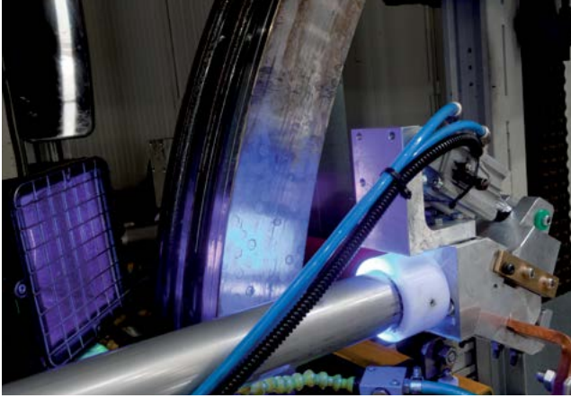
Magnetic particle crack check
