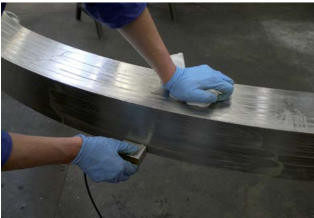
Ultrasonic material defect test
