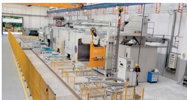
Zinc coating and paint automatic transfer machine
